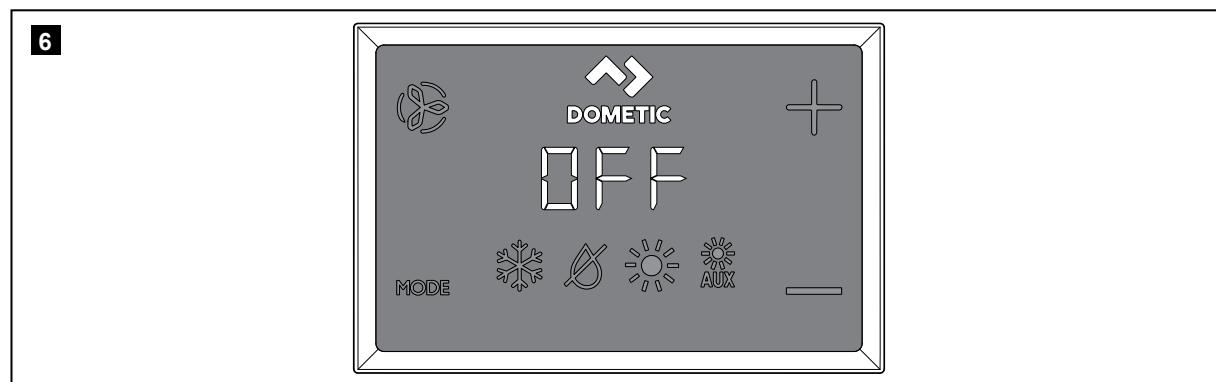
The four mode icons indicate the different modes of the control: COOL, MOISTURE, HEAT, and AUX HEAT. Refer to "6.3 Using the control panel" on page 11 for more detail on mode operation.
