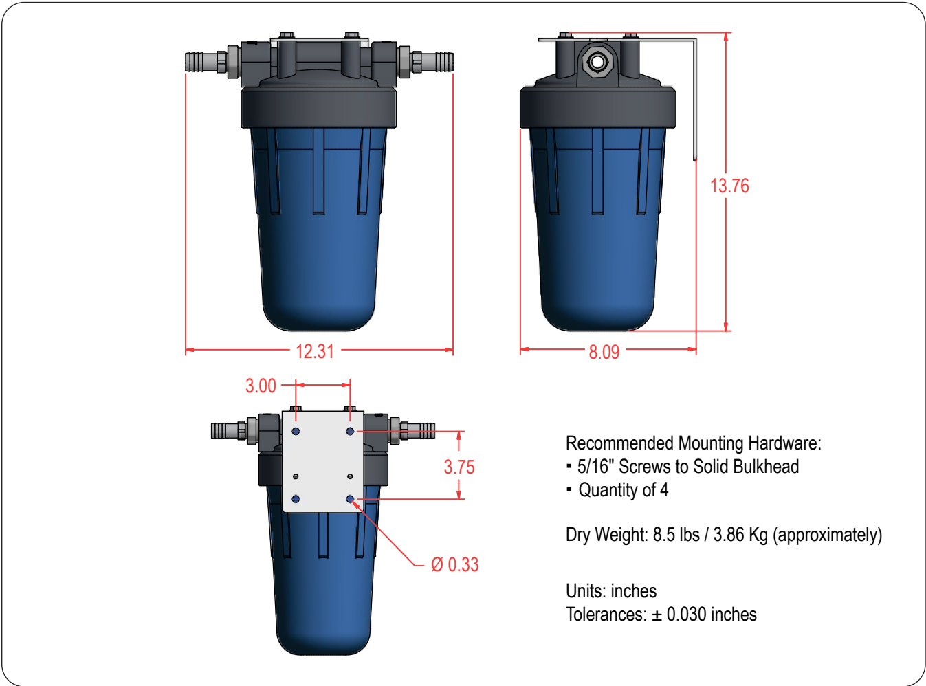
Figure 7: Dimensions Carbon Inlet Filter (P/N 93-5371)
