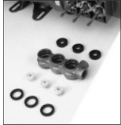
Plunger, Seals and V-Packing Arrangement
