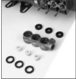
Plunger, Seals and V-Packing Arrangement
